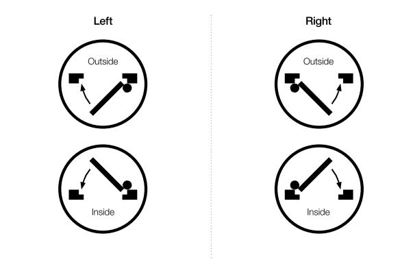
**Inside** (angle of the spindle in assemblies of 4A = ABLOY 4190 or LC 204)
