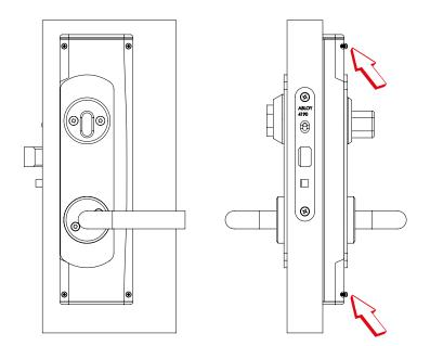
After installation, two of the short screws shall be replaced with the longer ones, which are screwed into the door and fixing the Duo unit.
